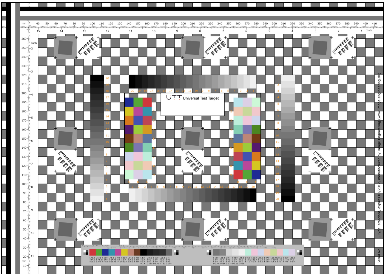
A representation of the Universal Test Target designed according to this specification.
